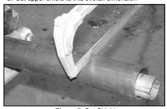
Figure 5. Cut Shield
